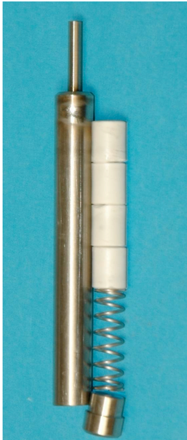
Halfniium Oxide surrogate fuel rod.
